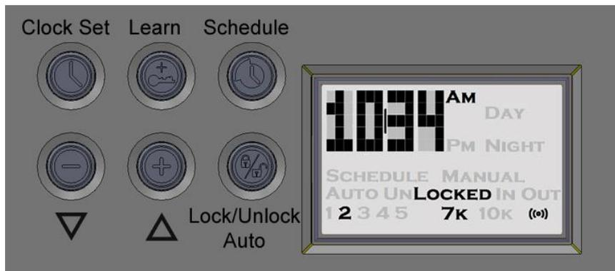
*Figure 1: Pushbuttons for Controlling Door Functionality*
