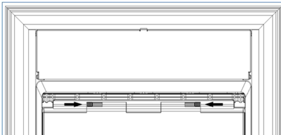
Reinstall the Doorman™ flap by inserting one of the locking pins into the mounting bracket. Slide the adjacent spring tab until locking pin is flush with flap edge. Carefully insert the flap into the frame aligning the locking pin into the mounting bracket.
